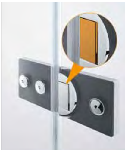
NEW TECHNOLOGY: The rise & fall mechanism - now discreetly hidden behind a cover - gently lifts the door on opening. This spares the lower seals and enables almost automatic closing of the doors
