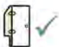
Slopes at the top or right-angled cut-outs at the bottom are possible in the fixed segment only.
