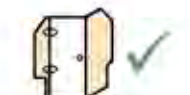
Sloping cuts for a sloping ceiling at the top or right-angled cut-outs at the bottom in the fixed segment and the side panel are possible.
